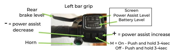
7) Ensure the power e-assist indicator displays 'low'
